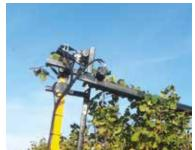
One movement topping device Our one-movement topping device is designed for extensive orchard systems without support posts. The angle
