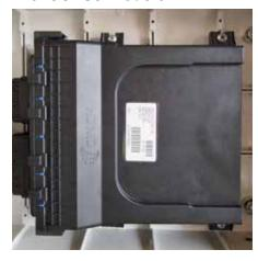
The ISOBUS connector for connection to the tractor
